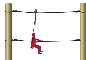
HIGH CHAIR: Participant sits on chair connected with a pulley to a cable and pushes himself across using a rope hand line
